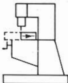
Cross feed table movement from front to back should display (-) directional count on "Y" axis
