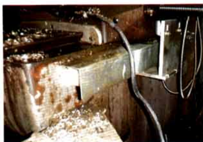
Right method: Use chip/coolant covers as shown above.
