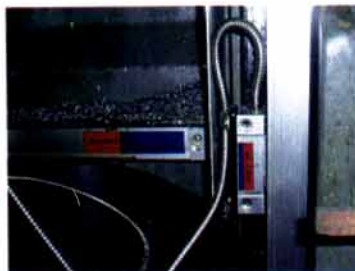
Wrong method: The glass scales are exposed to chips!
