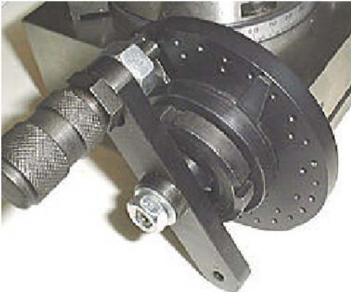
Sector arms set to advance 4 extra holes on the 28-hole circle.
