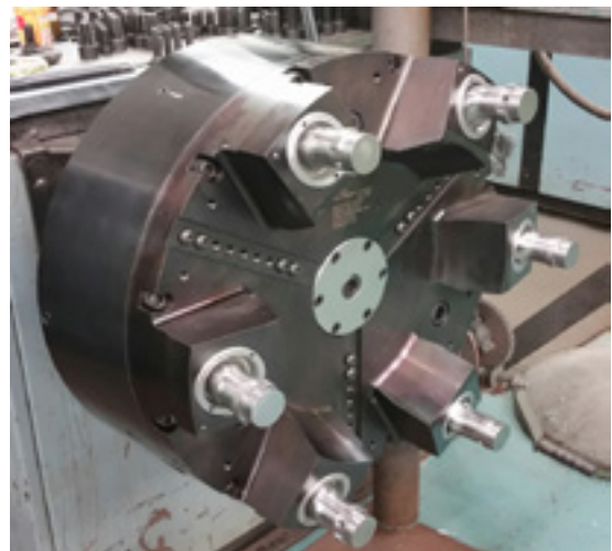
24" PC Chuck used for holding semi-truck brake drums.
