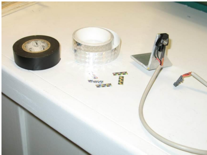
Example IR Reflective Bracket Mounting and Tape Patches
