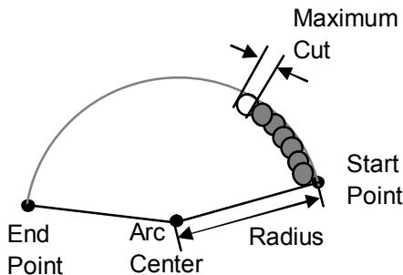
This function calculates the positions of points along the line of the arc using the required parameters.
