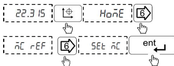
Move the machine to the required machine reference position. Then navigate with left/right arrow key to Set Machine Reference menu and press Enter to confirm the position.
