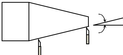
Taper function allows user to calculate taper of the job. Measurements carried out in Taper function are Radius of taper and Angle  $\theta^\circ$  of taper. Taper on axis setting is available in DRO setup menu. This will select where to display taper angle. See [Section 6.2](#).
