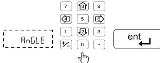
Enter **angle of grid** with positive X axis between two holes.
