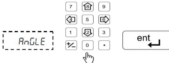
Enter **angle of line** with positive X axis between two holes.
