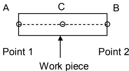
**Center Of Line** function allows user to find center of a line by locating end points of the line. Distance to the center from current location is shown on DRO display as **Distance-to-go**.
