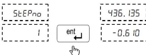
Enter the required step number on  $\text{Y}$  axis display. Press Enter to confirm.
