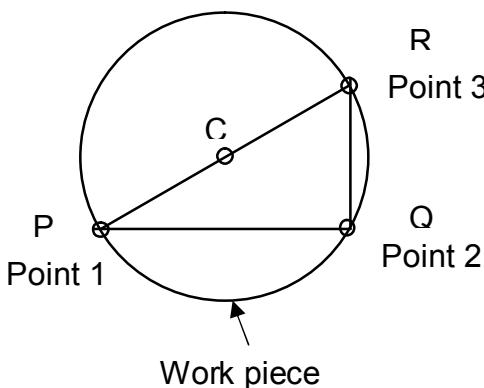
**Center Of Circle** function allows user to find center of a circle by locating three points on the circle.
