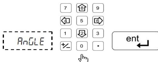
Enter **starting angle** this angle is with positive X-axis.
