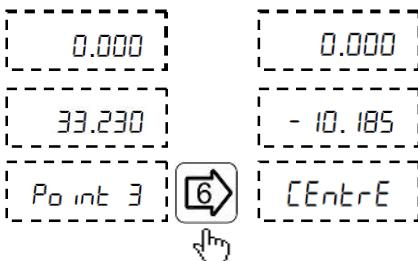
After storing all three points press to display **Distance-to-go** to center of circle.
