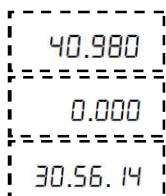
Now move the tool to the other end of the taper. Taper angle is displayed on DRO display.
