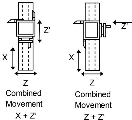
Axes Summing function is used to display combined movement of either X – Z axes pair or Y – Z axes pair. The summing axis pair can be displayed either on X axis or Y axis. Summing pair axis configuration setting is available in DRO setup menu. See [Section 6.2](#)
