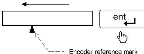
Move the machine to cross reference mark and reach the start point of the first segment.
