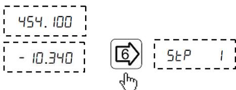
Move the machine to the position to be stored as sub datum for all axes and press  $\text{[6]}$ . This will show the current step number. By pressing the  $\text{[6]}$  again will store the position and go to the next step.
