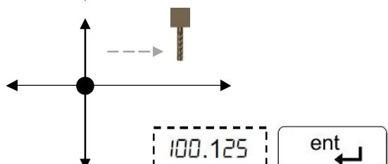
Move the axis away from datum point to put the slip gauge at datum point.
