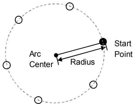
**Circular Bolt-Hole** function (also known as PCD) allows user to generate a pattern of holes along the perimeter of circle. After taking data from user such as co-ordinates of centre, radius, starting angle and number of holes, the table of required points is automatically generated and user is shown distance required to travel to each hole.
