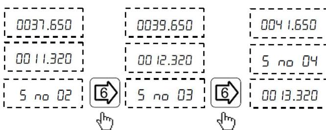
Using left and right keys user can go through all segments.
