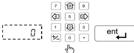
Input the reference value of slip gauge in **millimeter (mm)** and press
