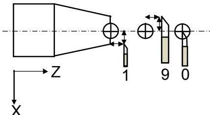
Tools differ in length as well as in diameter, making compensation in slide movement necessary to accommodate the dimensional variation of the tools. This compensation is known as the tool offset. Once the tool offset is established, the slide movement is automatically adjusted according to the value that is set. MNEL 400 series DRO supports 9 such tool offsets.
