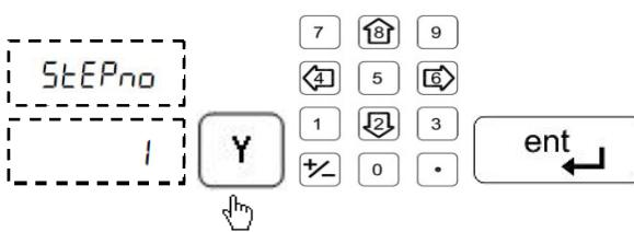
As a standard step number 1 is displayed. This can be edited by pressing **Y** axis key and entering the required step number.
