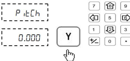
Reset axis by pressing axis key. Enter the required pitch and press
