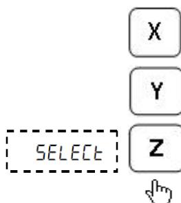
Select axis along which Linear Bolt Hole pattern is to be generated.
