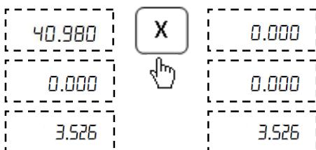
Touch the tool to one end of the taper and reset X and Z axis.
