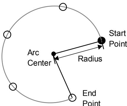
Arc Bolt Hole function is very similar to Circular Bolt Hole function, except in arc hole function user can enter the starting and ending angle of an arc. This angle is always with respect to positive X-axis and is calculated in anti-clockwise direction.
