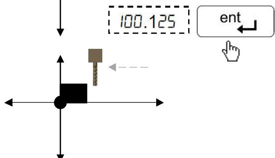
Move the axis to touch the slip gauge. The display value is the measured length of the slip gauge
