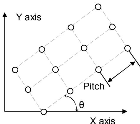
The grid function calculates the locations of the holes of pattern in XY plane. This pattern can be at a tilt angle from X axis. The calculations are done with parameters like starting point co-ordinates, holes spacing, tilting angle of the line and number of holes.
