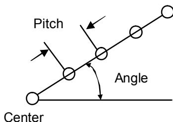
This function calculates the position of the holes on a line with the help of parameters such as starting point, pitch angle of a line and no. of holes.
