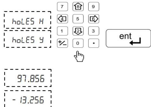
Enter total **number of holes** for X axis and Y axis.
