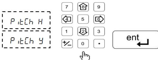
Enter distance between two holes for X axis and for Y axis.
