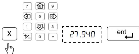
Select axis key. Enter the numeric value to preset the selected axis. Confirm with key.
