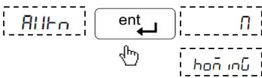
Last digit of axis display is blinking which indicates that this axis is ready for sensing the reference mark.
