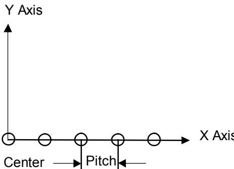
Linear Bolt Hole function allows user to create an equality spaced pattern of holes in linear direction. After taking data from user such as axis and pitch, the table of required points is automatically generated and user is shown distance required to travel to reach particular hole.
