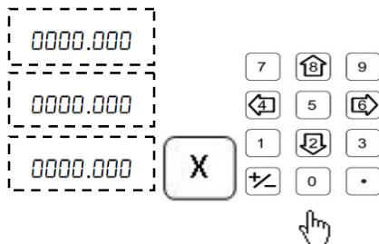
Select the required axis and enter the values for the selected step. Press
