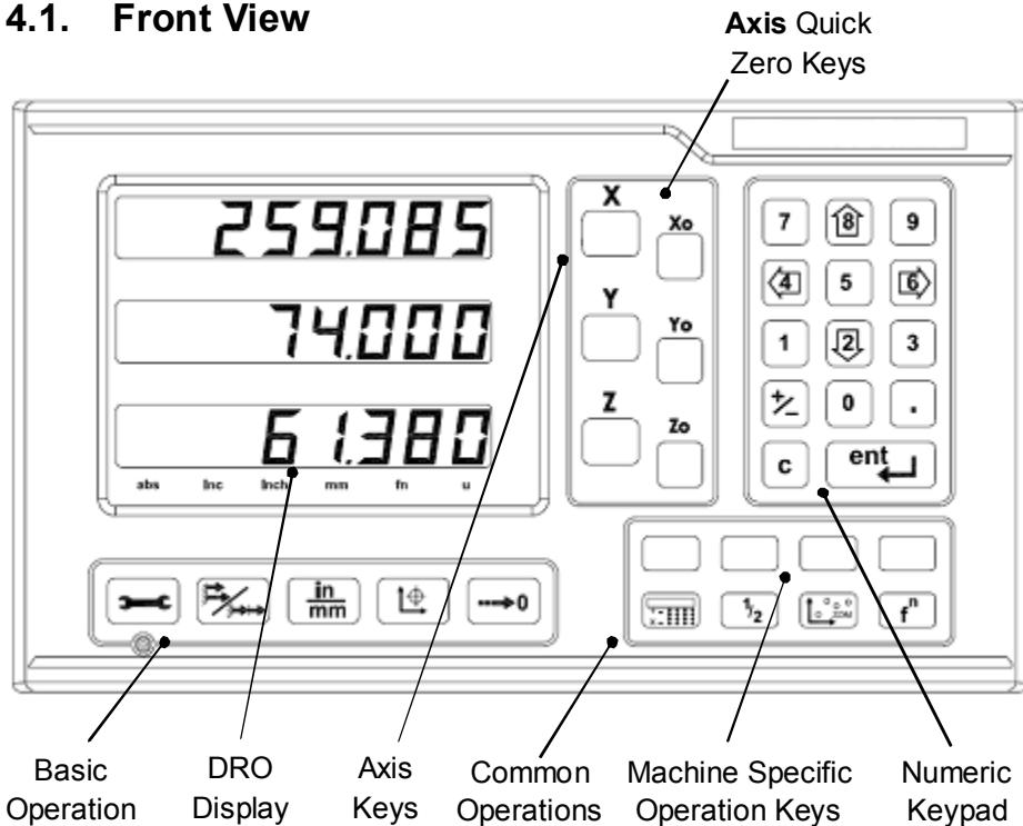
⚠ Note: In 4 Axes model, press Z followed by Z0 to toggle between Z and U axis display.
