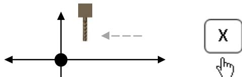
Set the machine at datum point (starting point) and press the axis key to reset the axis.
