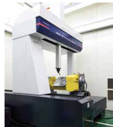
Accuracy measurement with large 3 Dimensional Measuring Machine
