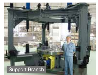
CNC1800 & Support Branch Indexing/ clamping of the turbine disk
