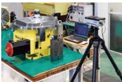
Indexing Accuracy Measurement by Laser
