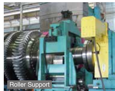
CNC1201 Indexing of the turbine shaft. Turbine shaft is supported and clamped by the roller support.
