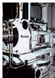
CNC401T is installed on CNC600.
