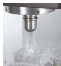
CCK collet & CCKFN nut The Jet Coolant Pressure creates a tornado effect, ensuring efficient swarf dispersal.
