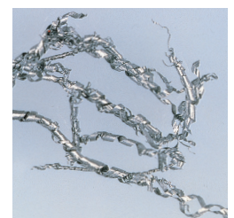
Swarf by reaming blade
