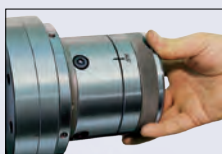
Clamping with collet and longitudinal workstop
