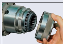
Clamping with collet and longitudinal workstop
