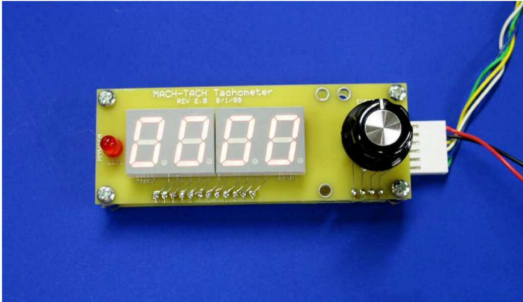
Completed Half Size Module (older revision PCB with side connector)
