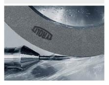
Cool grinding: The combination of innovative grain quality and adapted bonding system reduces the grinding forces and thus the temperature.
