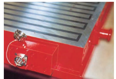
Waterproofed quick-connection for the cable
