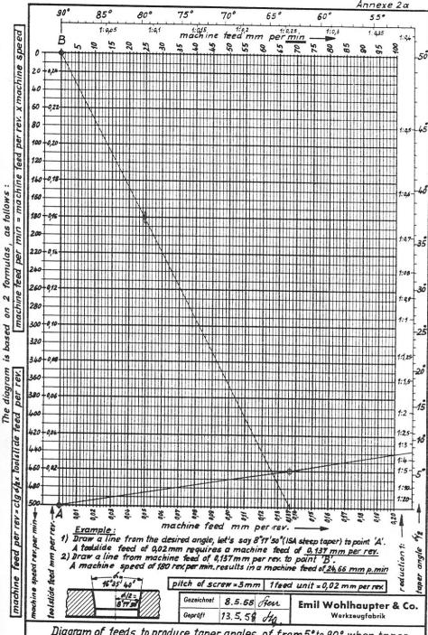
Diagram of feeds to produce taper angles of from 5° to 30° when taper turning with "WOHLHAUPTER" Facing and Boring Heads UPA4... UPA657
