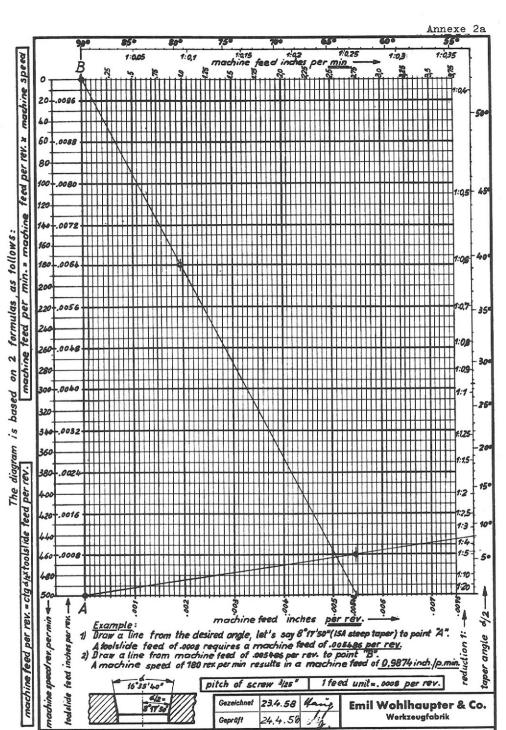
Diagram of feeds to produce taper angles of from 5°... 90° when taper turning with "WOHLHAUPTER" Facing and Boring Heads UPA4...UPA6-57
