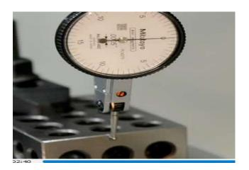
**Step 10** Enter the readout after the decimal point as the axis CPI.
