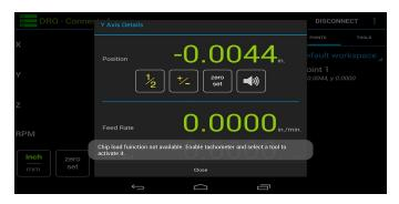
\*Setups that don't include a tachometer can still take advantage of this function by entering the RPM directly using the "Set RPM" function as in **Section 4**.
