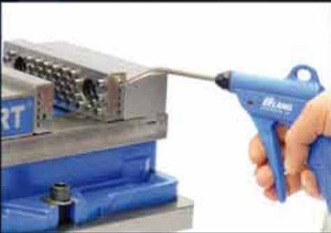
Pins are extended by compressed air
